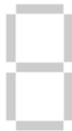
FIGURE C.1: Numeral frame also known as the seven-segment display
